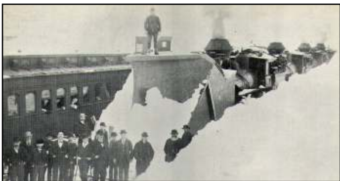
A bucker plow at Cisco. (Ken Yeo Collection) These were pushed through drifted snow by several locomotives, as shown in the lower photo taken at Blue Canyon in 1890. Derailments were a frequent problem. (Lower photo from Best – Snowplow)
