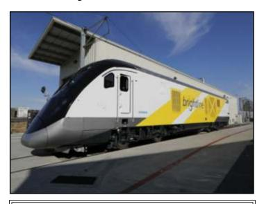
Brightline's first Siemens Charger diesel-electric locomotive has successfully completed initial testing and operated for the first time, powered by its Cummins QSK95 diesel engine, on the quarter-mile test track at the Siemens manufacturing facility in Sacramento, Calif.
