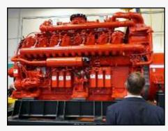
This Cummins 16 cylinder 4000HP diesel engine is being installed by Siemens in its Charger locomotives. See page 3 for brief recap of PSRHS field trip to Siemens' facility. Photo from USA Today.
