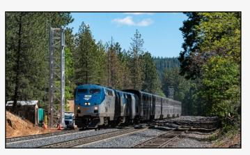
AMTRAK #5 passes a support truss for one of the cantilever signal bridges being installed as part of the new high speed crossovers at Gold Run. See photos and story on pages 3-4. Paul Greenfield photo
